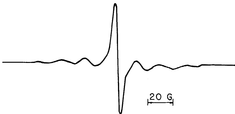
Figure 4. EPR spectrum of \gamma -irradiated glassy MTHF at 73°K (dose 0.5 Mrad).
